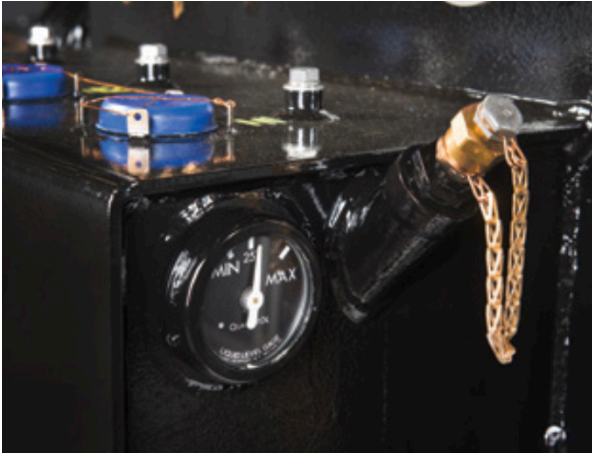
Switch-box liquid-level gauge and filling provision
