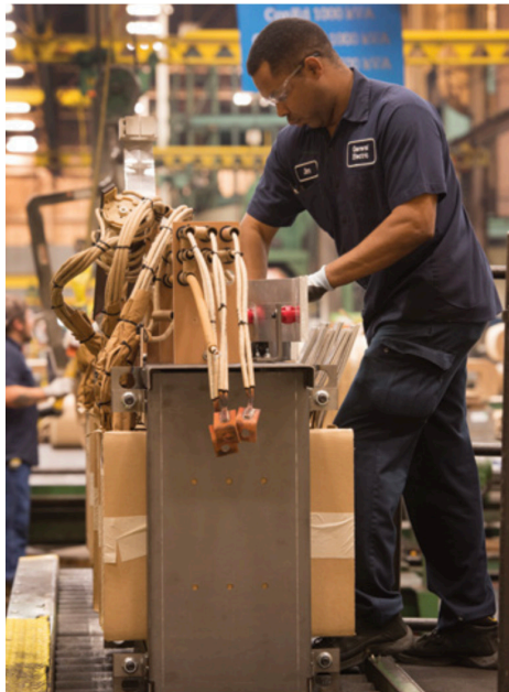
Assembly of Interior cabling and barwork
